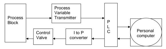
The SCADA-PLC instrumentation system for Multiple Effect Spent wash Evaporation plant is to be provided with UPS (Back-up for PLC room should be 1 hr. capacity) & printing arrangement. Automatic data storage for minimum 3 months period. This is to be placed in AC room & AC to be provided by the supplier to maintain the temperature of AC room in the range 20-25° C.
